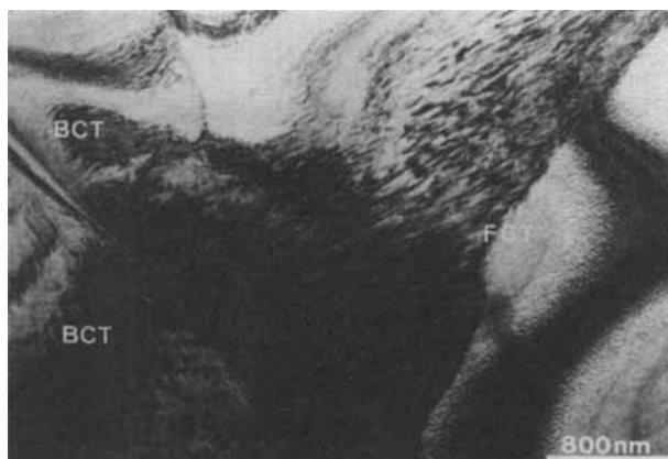
Fig. 7 The stress-induced f.c.t. phase observed near the austenite-b.c.t. martensite interface at 130K is shown (specimen No. 3)
