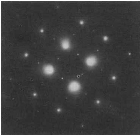
**Fig. 5(a)** The (001) type electron diffraction pattern for a palladium-12.5 atomic per cent yttrium alloy aged for one week at 475°C shows the superlattice reflections corresponding to a highly ordered structure
