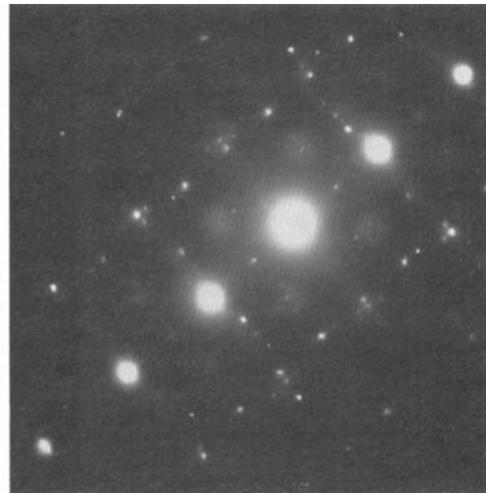
**Fig. 7** The light micrograph of partially retained  $\beta$  phase in a Ti-37Al-5Ru alloy quenched from a temperature of 1250°C is supplemented by an electron diffraction pattern and key, showing the Burger's type transformation
