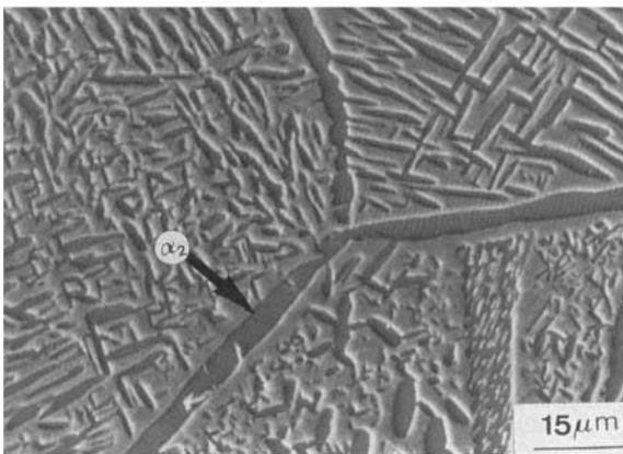
**Fig. 3** Fine scale  $\alpha_2 + \beta$  structures occur in Ti-18Al-5Ru quenched from a temperature of 950°C; an  $\alpha_2$  region is indicated on this SEM micrograph
