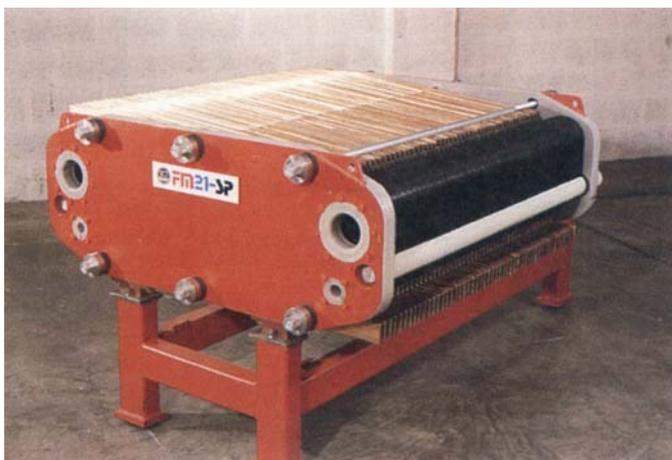
**Fig. 1** This electrolyser manufactured by ICI for the production of chlorine shows a typical modern compact cell which could be used at the heart of the process for the destruction of industrial organic waste materials
