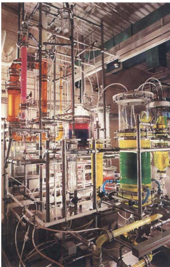
**Fig. 2 The pilot plant built at Dounreay for the destruction of organic waste is being used to establish the chemical engineering parameters that are required for a full scale plant**
