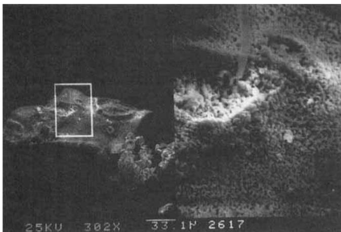
**Fig. 5** This large irregularly shaped particle with a highly altered surface, recovered from the catalyst gauzes, consists essentially of iron. All the features suggest that it originated from part of the reactor wall, and had been degraded by the arduous operating conditions
