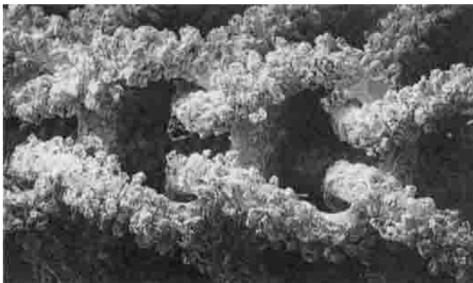
Fig. 3 After commercial trials under atmospheric conditions, excellent surface development was evident on a knitted gauze, and this extended to areas of potential masking × 100 approx.
