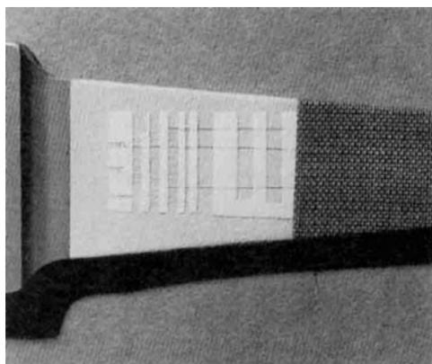
**Fig. 3** After the application of an alumina precoat, the compensated wire gauge is taped down with high temperature adhesive strips. Here the substrate is an IN-718 test bar
