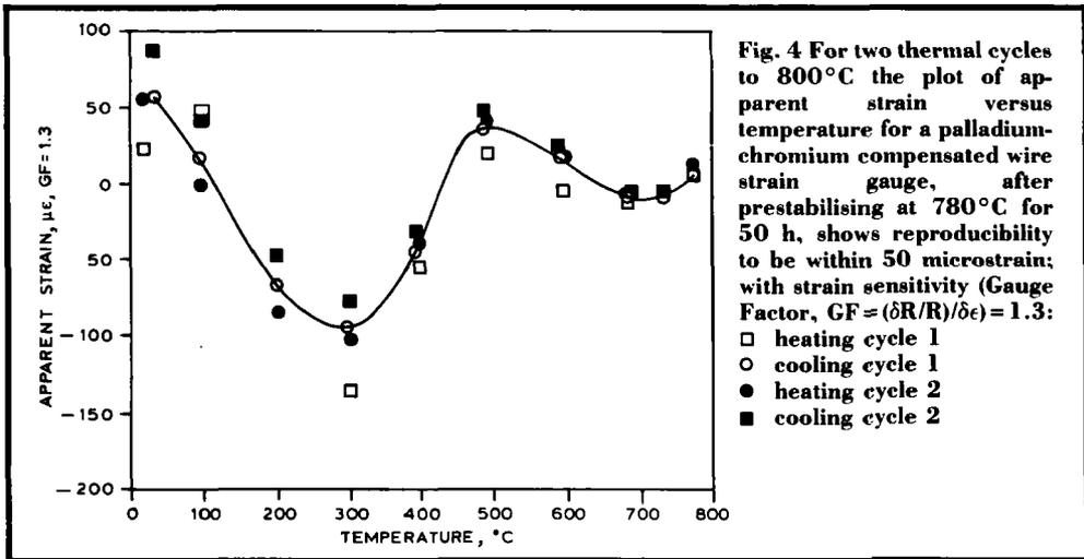
room temperature to 800°C is within 300 microstrain ( $\mu$  inch/inch), with a reproducibility to within 50 microstrain between thermal cycles to 800°C, see Figure 4. The apparent strain of the gauge can therefore be corrected at temperatures up to 800°C, due to its small value and its repeatability. This is a significant advance on the previous techniques for existing static strain gauges, as demonstrated by the data in Figure 5.
