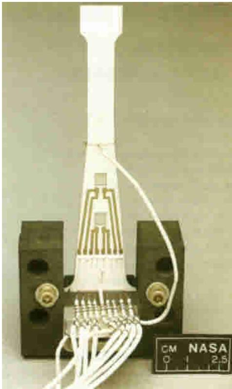
**Fig. 6** These two sputtered thin film gauges, on an alumina test beam, were produced as part of a NASA development programme. The enlargement below shows details of the palladium-chromium thin film gauges
