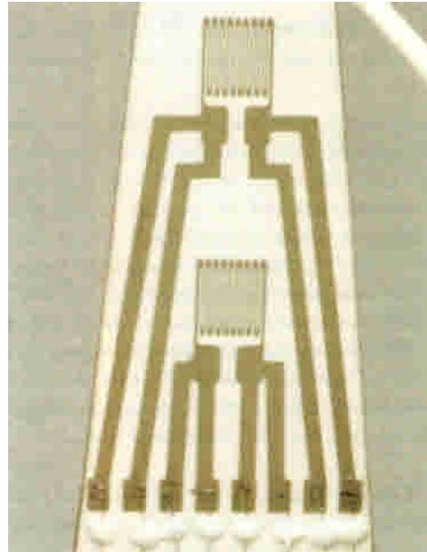
the thin film lead pads. The apparent strain change versus temperature characteristics of these sputtered thin film gauges is linear and repeatable at temperatures up to 1000°C. The reproducibility of the apparent strain between repeated thermal cycles to 1000°C can be further improved by prestabilising the gauge before testing, and by coating the gauge with the
