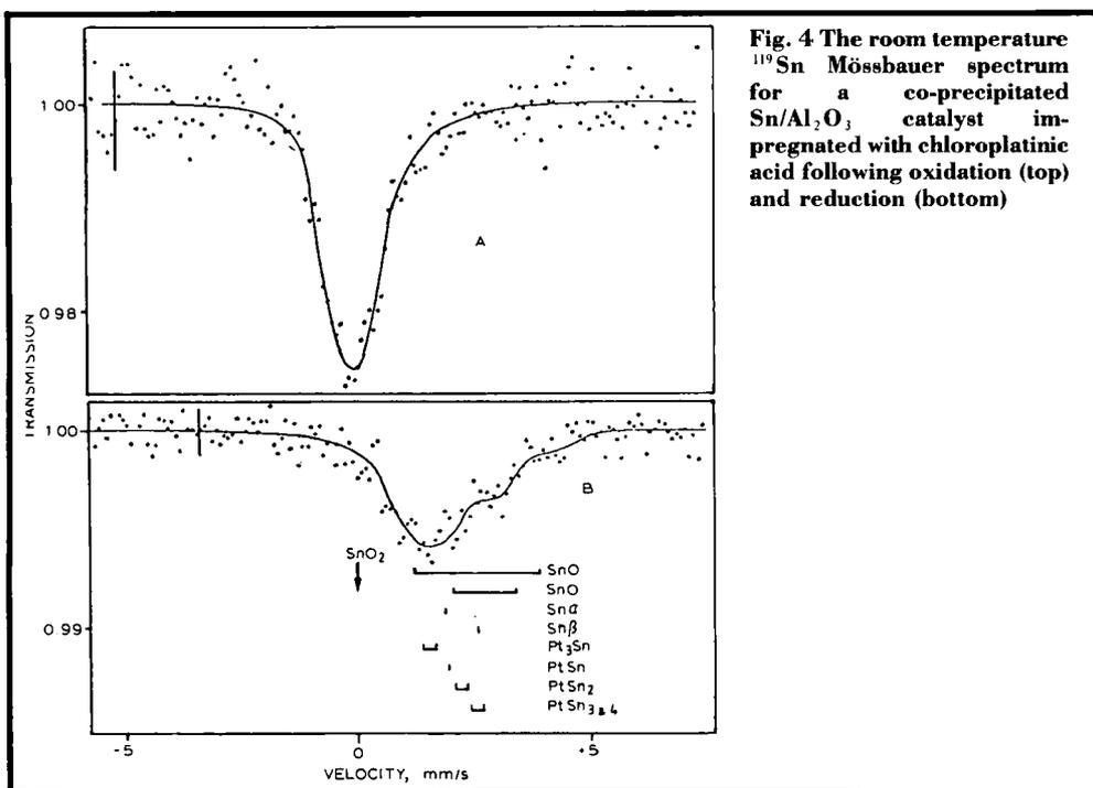
Fig. 4 The room temperature  $^{119}\text{Sn}$  Mössbauer spectrum for a co-precipitated  $\text{Sn}/\text{Al}_2\text{O}_3$  catalyst impregnated with chloroplatinic acid following oxidation (top) and reduction (bottom)
