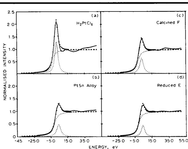
Fig. 10 Profiles at the Pt  $L_{III}$  edge, resolved into overlapping Lorentzian and  $\tan^{-1}$  functions. The large dots show how well the recorded data (—) are reproduced by the sum (....) of the functions (.....)
