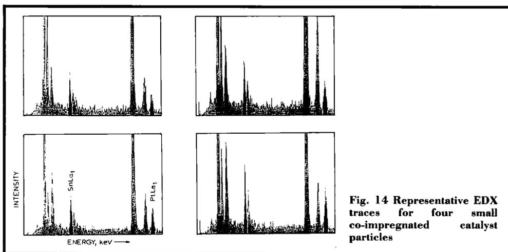
**Fig. 14 Representative EDX traces for four small co-impregnated catalyst particles**
