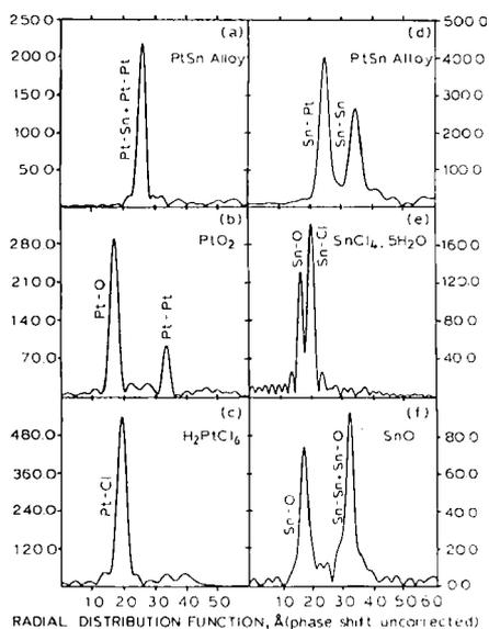
Fig. 11 Radial distribution functions derived for the calibrating materials; (a), (b), (e) at the platinum  $L_{III}$  edge, and (d), (c), (f) at the tin K-edge
