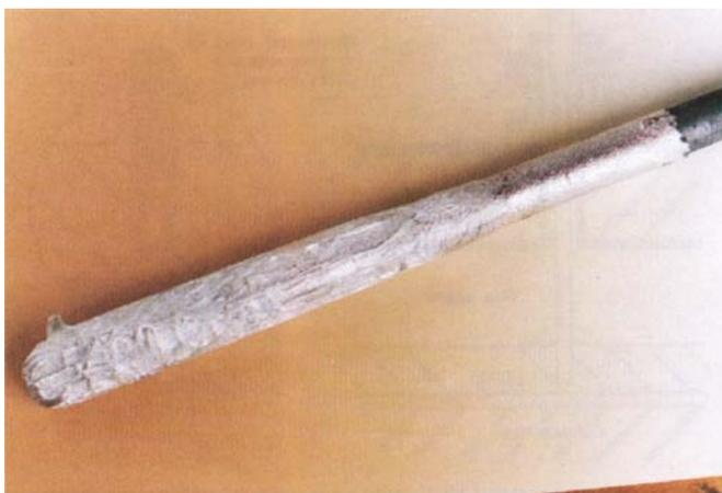
thermal stabilities at high temperatures. Considerable laboratory testing of such coatings was undertaken before the work was extended to include field trials of protected nickel-chromium alloys. This work was performed in forehearths of major glass container companies in the U.K. and in Australia. With typical molten glass temperatures of between 1100 and 1200°C, substrate protection was achieved for up to the maximum test time of 4500 hours, Figure 5.
