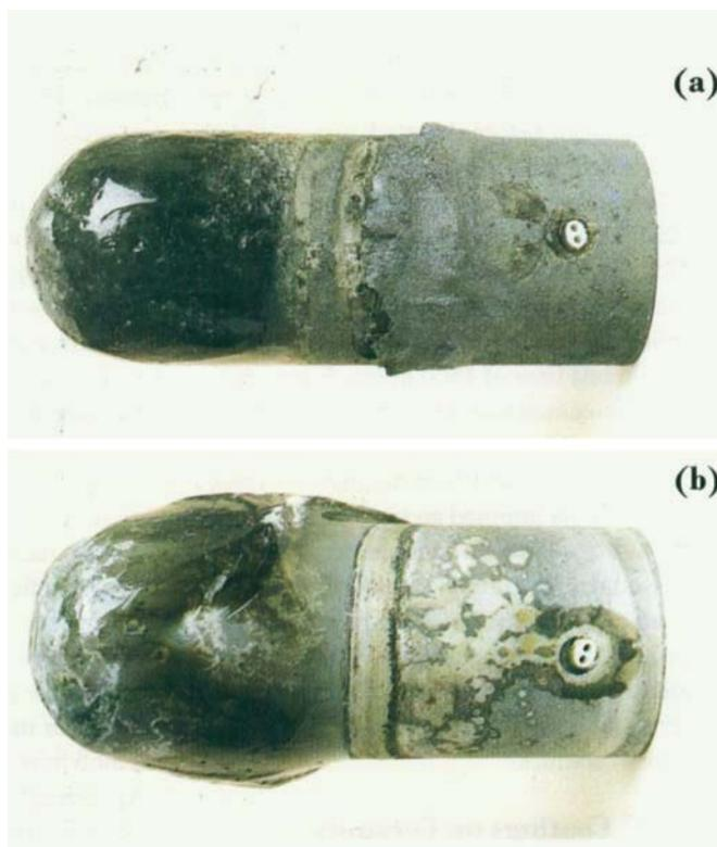
constituents of the outer protective coating and the underlying substrate material. Such inter-diffusion is usually deleterious.
