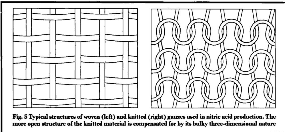
is generally believed that the campaign life may be extended by increasing the number of gauzes in a pack, so that contamination of the leading gauzes results in the transfer of the reaction zone to a greater depth, without causing any loss of efficiency. This does not happen, however, since the ammonia is less selectively oxidised to nitric oxide; instead more is oxidised to nitrogen as the level of contamination increases.
