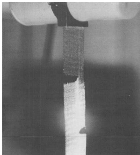
**Fig. 8** Although the herringbone structure is considered to be one of the strongest conventional weaves, a tensile test sample tore almost instantly when under load
