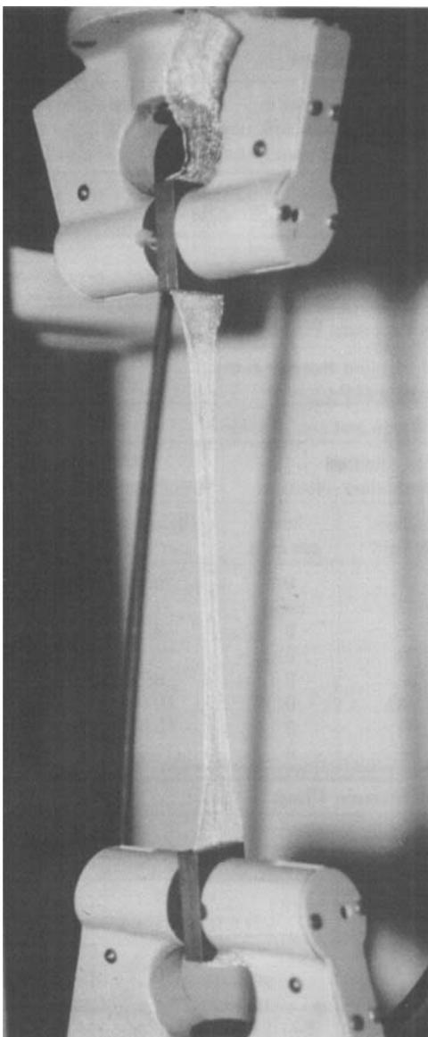
**Fig. 7** A tensile test sample of knitted gauze stretched significantly before fracture, which usually occurred at the clamping jaws
