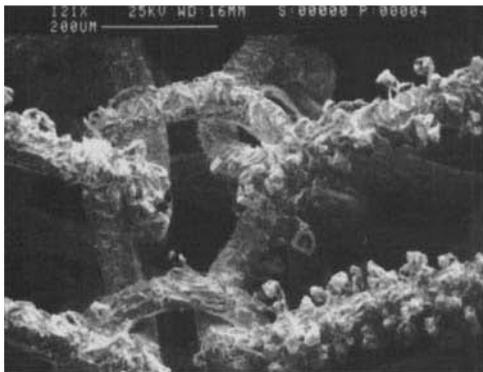
**Fig. 9** After use for ammonia oxidation both woven and knitted gauzes show restructuring of the surface. Fragile “cauliflower” like formations grow on both types of catalyst but on knitted gauzes the structural rearrangement is widely dispersed throughout the catalyst pack leading to a more even temperature distribution, less mechanical damage and reduced metal loss, compared to the woven gauze
