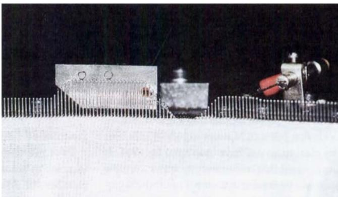
approximately 1990 needles around the circumference, see Figure 2, the size being determined by the need to reduce wastage and minimise seam fabrication. Having already determined the optimum density of the cloth on the earlier development machine, the needle spacing and stitch length were maintained to achieve continuity.
