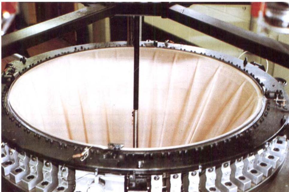
**Fig. 4** The four knitting heads are supplied with fibres at a computer-controlled constant rate to produce a knitted tubular gauze, of uniform tension and homogeneous density. The first production knitting machine was 76.2 cm in diameter and had approximately 1990 needles around the circumference
