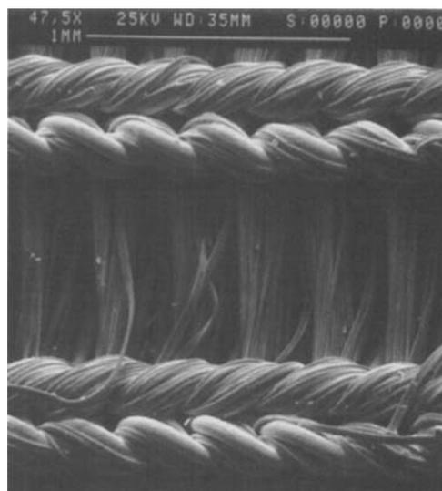
**Fig. 3 The carrier is a multi-stranded polyester fibre which almost completely covers the platinum alloy wire during the knitting operation. The carrier is removed after the gauze is cut to size and before the catalyst is activated for use**
