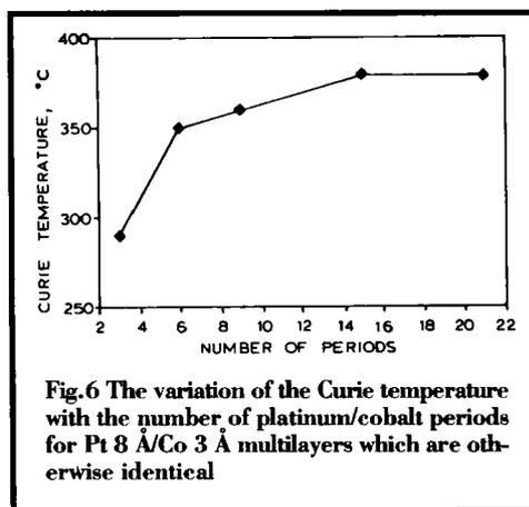
Fig.6 The variation of the Curie temperature with the number of platinum/cobalt periods for Pt 8 Å/Co 3 Å multilayers which are otherwise identical
