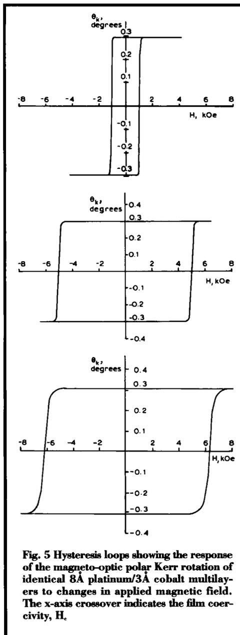
**Fig. 5 Hysteresis loops showing the response of the magneto-optic polar Kerr rotation of identical 8Å platinum/3Å cobalt multilayers to changes in applied magnetic field. The x-axis crossover indicates the film coercivity,  $H_c$ .**
