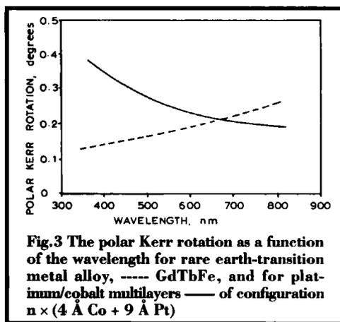
**Fig.3** The polar Kerr rotation as a function of the wavelength for rare earth-transition metal alloy, ---- GdTbFe, and for platinum/cobalt multilayers — of configuration  $n \times (4 \text{ \AA Co} + 9 \text{ \AA Pt})$
