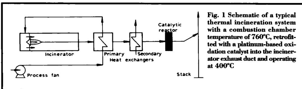
**Fig. 1 Schematic of a typical thermal incineration system with a combustion chamber temperature of 760°C, retrofitted with a platinum-based oxidation catalyst into the incinerator exhaust duct and operating at 400°C**
