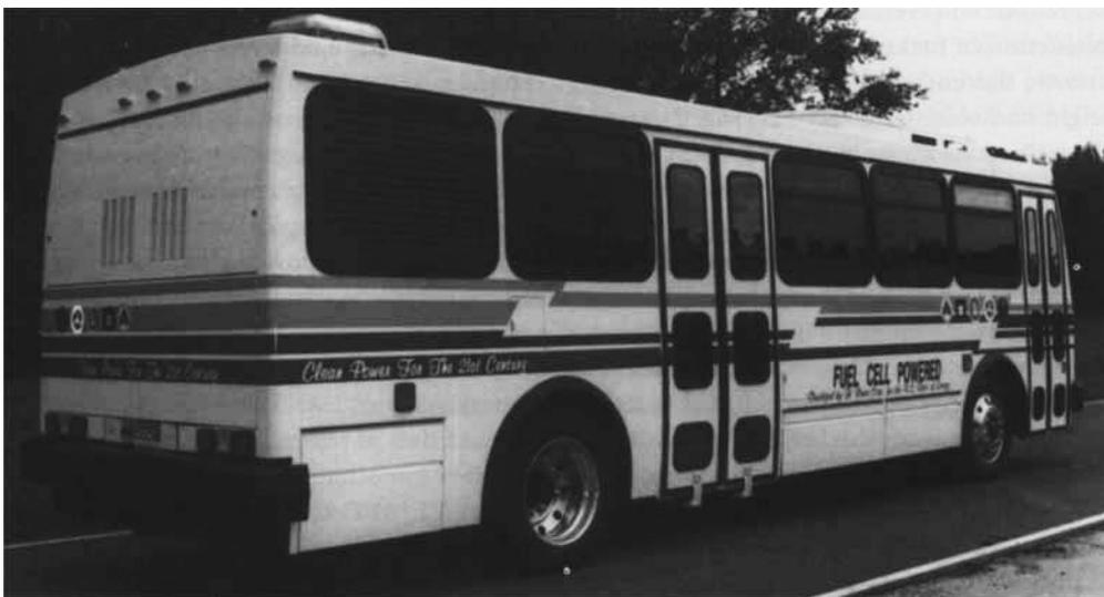
**Fig. 3** The first methanol-fuelled, phosphoric acid fuel cell powered transit bus, produced by H Power Corporation in the U.S. Department of Energy sponsored programme. This meets all the required performance criteria but with improved fuel efficiency and significantly reduced exhaust emissions and noise pollution
