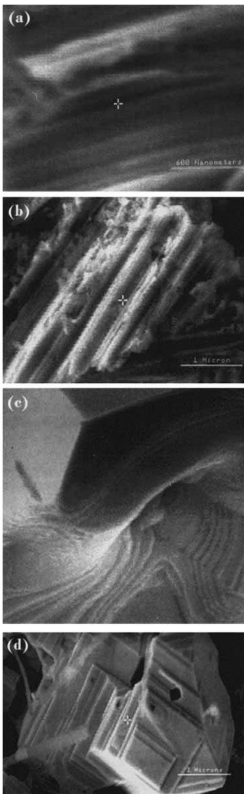
**Fig. 6** The layered structure that is observed during recrystallisation is controlled by a ladder-like growth process: (a), (b) and (c) are surfaces of (G-5)[c], (G-5)[b] and (G-5)[a] of (G-5) gauze, respectively, and (d) is the [c] surface of (G-8) gauze
