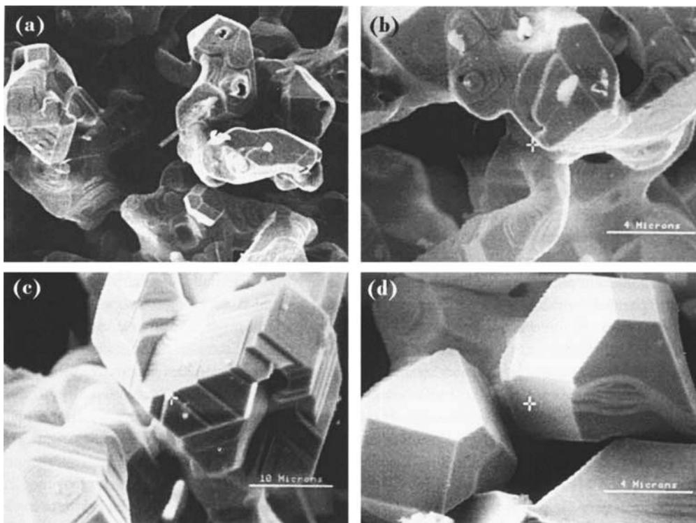
Fig. 7 Screw growth and screw cones occurring during recrystallised crystal growth: (a) the (G-8)[c] surface; (b) the (G-8)[b] surface, showing screw-type growth and screw cones; (c) the (G-8)[b] surface, showing ladder-like structure and small screw cones on the crystal face, and (d) the (G-8)[a] surface for (G-8) gauzes
