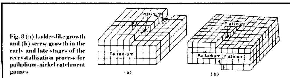
Fig. 8 (a) Ladder-like growth and (b) screw growth in the early and late stages of the recrystallisation process for palladium-nickel catchment gauzes
