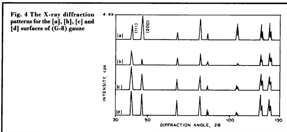
of (G-5) and (G-8) gauzes are larger than those of palladium-5 per cent nickel alloy and pure palladium. Thus, the solid solubility of platinum, which has a larger atomic radius (0.139 nm) than palladium (0.137 nm), increased in the palladium matrix, while the solid solubility of nickel in palladium decreased. That is to say, the initial solid solution of palladium(nickel) has transformed gradually into a palladium(platinum) solid solution, while the catchment gauzes were in use.
