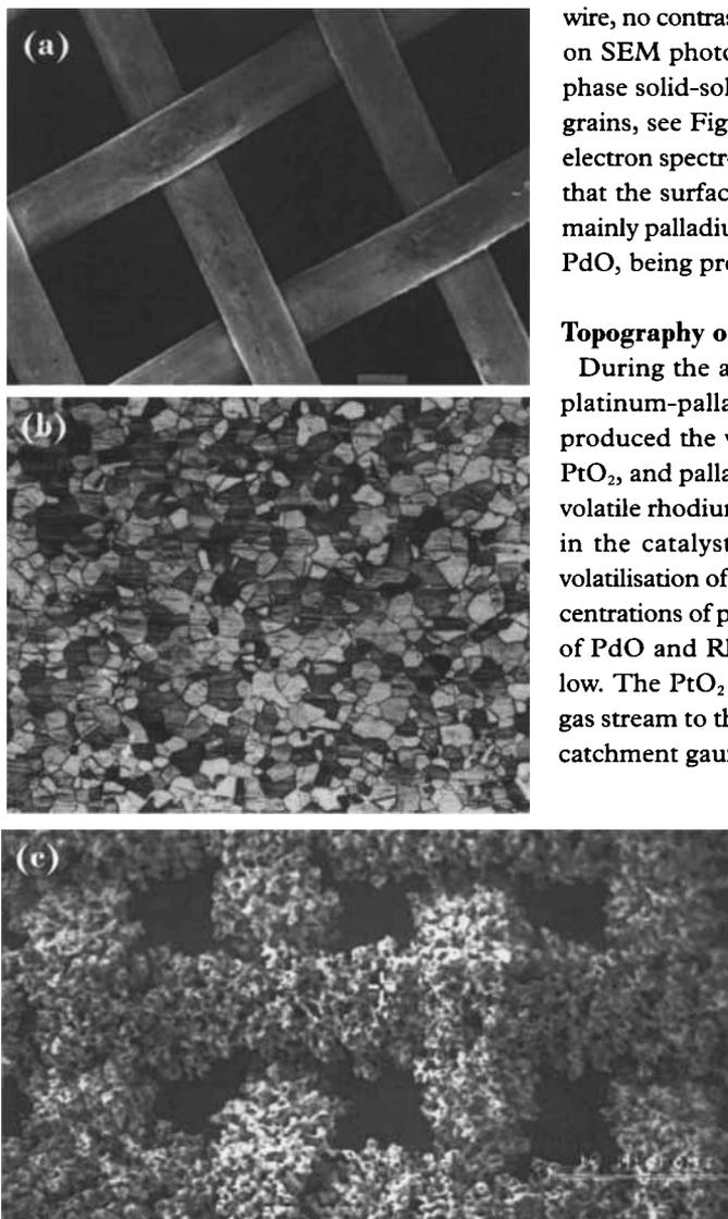
**Fig. 1** Fresh palladium-5 per cent nickel catchment gauzes showing: (a) the surface topography, the scale line is 100  $\mu\text{m}$  (b) the crystal structure, and (c) the surface topography of (G-5) gauze, after being used for 5 months; the line is 10  $\mu\text{m}$  long
