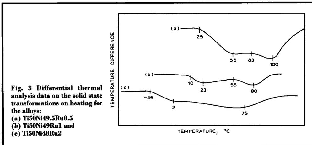
**Fig. 3** Differential thermal analysis data on the solid state transformations on heating for the alloys:
