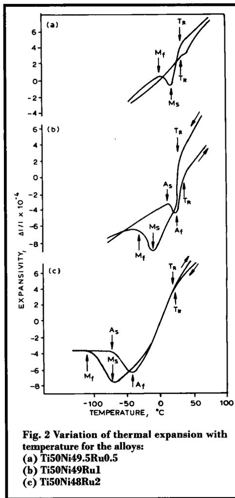
**Fig. 2** Variation of thermal expansion with temperature for the alloys:
