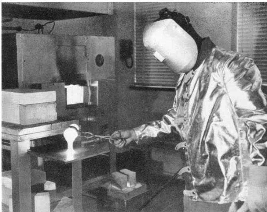
*A laboratory worker at Corning Glass Works, Corning, New York, pouring a sample of a new glass composition from a platinum-lined crucible*
