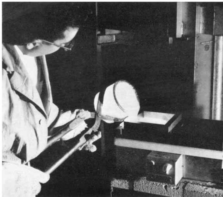
*Optical glass is produced by Bausch and Lomb of Rochester, New York, both in continuous-flow furnaces, portions of which are lined with platinum, holding 5 to 8 tons of glass, and in platinum-lined crucibles each holding up to 200 lb of glass. The platinum-lined pot shown here is pouring a small experimental batch of optical glass*
