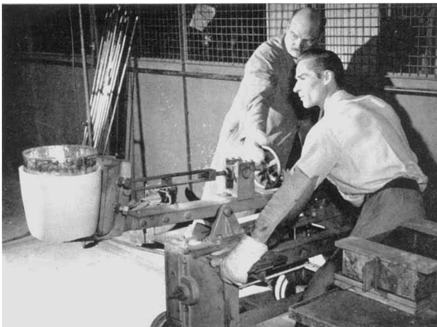
*Removing a platinum pot, supported in a refractory crucible, from the furnace at the Birmingham works of Chance Brothers Ltd. The pot holds 12 litres of optical glass*
