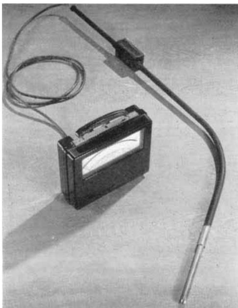
*For the measurement of temperature in molten glass, this platinum : rhodium-platinum thermocouple has been developed by the Foster Instrument Co. Ltd. The former refractory sheath has been replaced by a platinum sheath*
