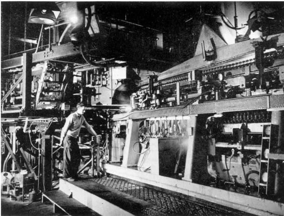
*Accurate temperature measurement and control are vital in the operation of modern glass-forming machines. This "ribbon" machine produces more than one and a quarter million electric lamp bulbs a day at the works of Glass Bulbs Ltd. at Harworth, Yorkshire, where more than fifty platinum thermocouples are installed*
