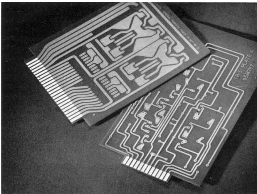
*Two printed circuits by Ferranti Ltd., designed for plugging into fixed sockets. The contact surfaces are palladium plated*
