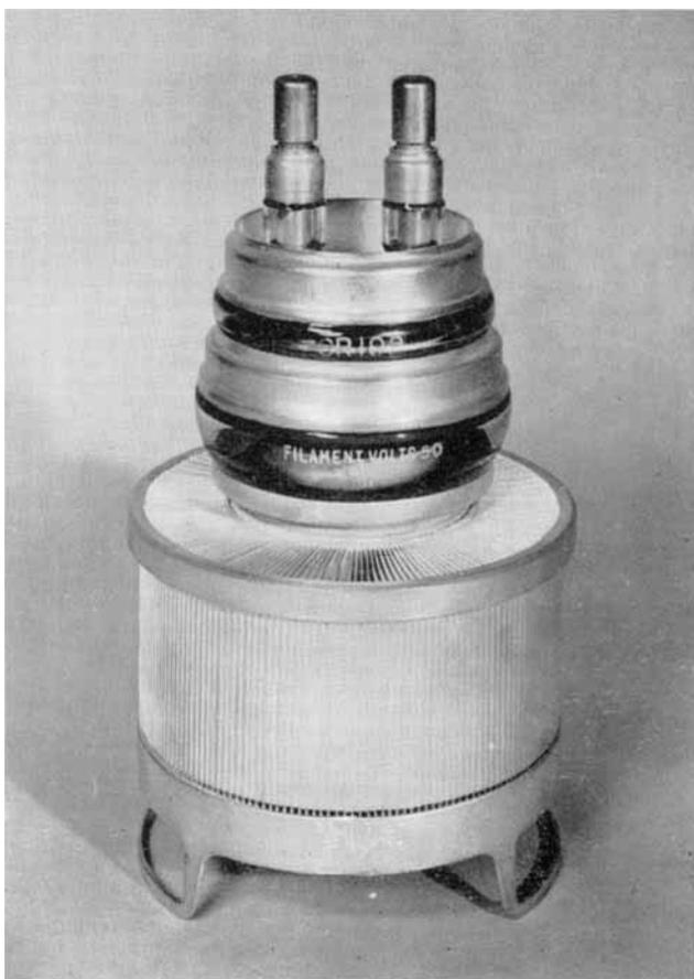
*A high-power television tetrode in which both control grid and screen grid are made of platinum-clad molybdenum wire*
