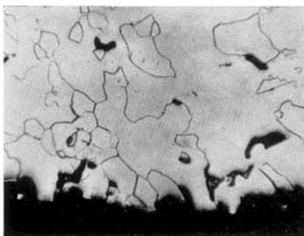
*Fig. 6 Fracture of recrystallised iridium showing the presence of intergranular failure  $\times 75$*
