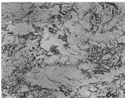
*Fig. 2 Iridium in the as received condition
