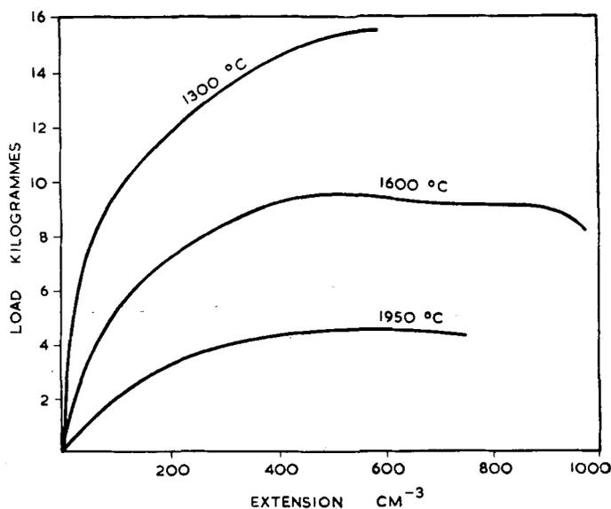
Fig. 3 Typical load-extension curves for iridium specimens
