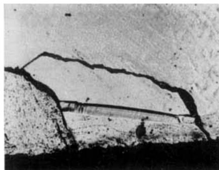
*Fig. 8 Twinned region in a recrystallised iridium specimen  $\times 94$*
