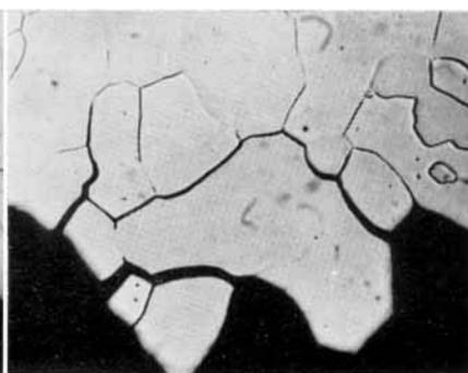
*Fig. 7 Intergranular fracture of iridium at 1600°C  $\times 75$*
