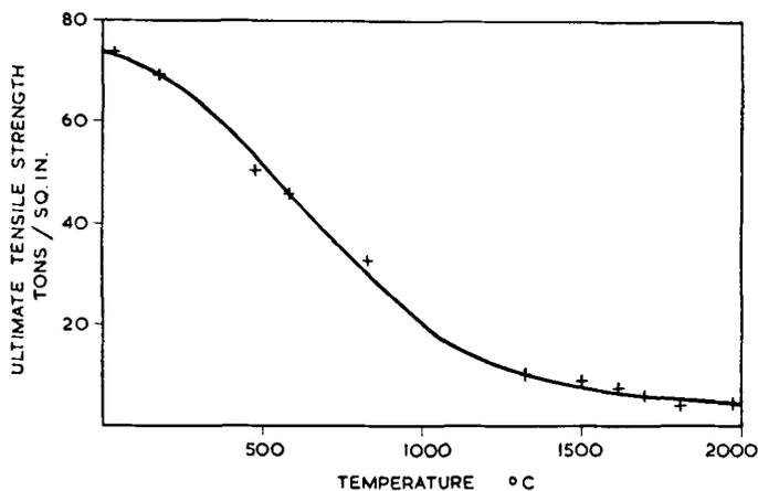
Fig. 4 Ultimate tensile strength of iridium as a function of temperature
