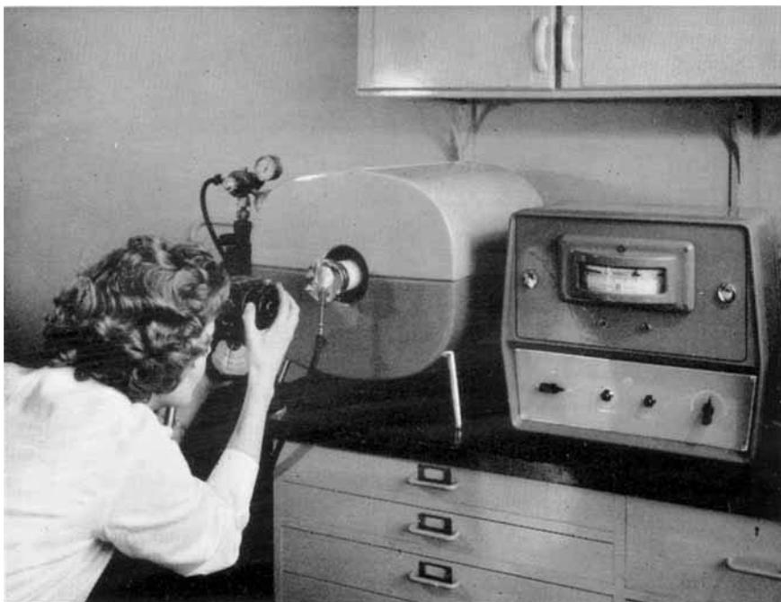
*Observing the fusion characteristics of a sample of coal ash in the Johnson Matthey platinum-wound furnace specially designed for this determination*
