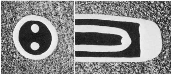
*Photomicrographs of the cross-section and longitudinal section of the hot junction show that the thermocouple wires are completely insulated from each other and from the sheath*
