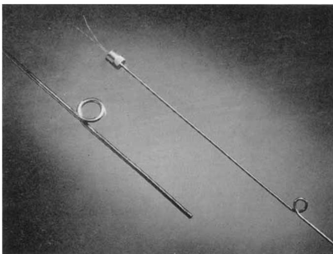
*This photograph of the two standard sizes of the Johnson Matthey metal-sheathed mineral-insulated thermocouple shows both the flexibility of assembly and the special end cap provided for the cold junction*
