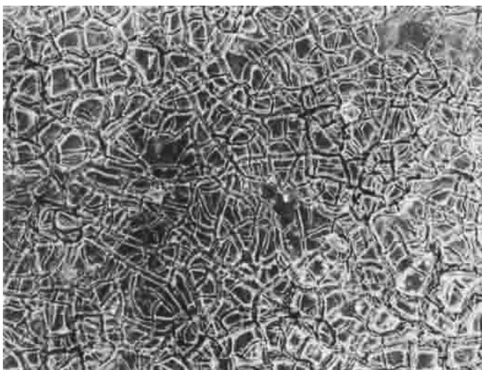
**Fig. 1 Scanning electron micrograph of a modern oxide coated titanium anode for a chlor-alkali cell. Scale: 1 cm represents 20  $\mu\text{m}$**
