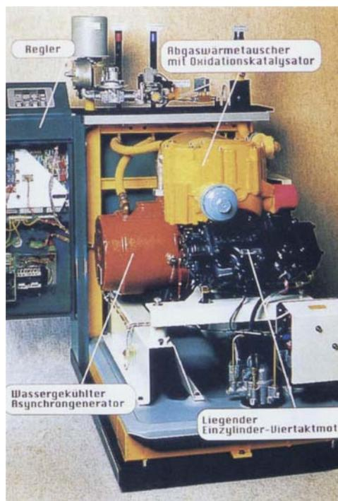
The co-generation unit showing the control console and the water-cooled heat exchanger where the emission control catalyst is situated
