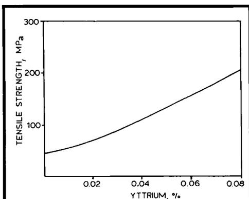
**Fig. 1 Relationship between tensile strength of platinum and its yttrium content at room temperature**
