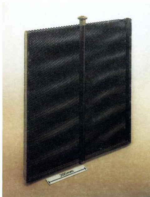
Fig. 7 A box-type diaphragm-type chlorine cell anode structure consisting of noble metal oxide coated titanium mesh spot welded to a central copper cored titanium rod and plain titanium sheet gussets
