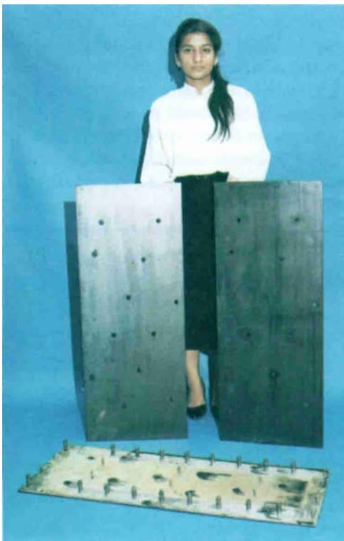
**Fig. 15** Typical titanium electrodes used in electrogalvanising plants. The laboratory assistant shows the size of such electrodes
