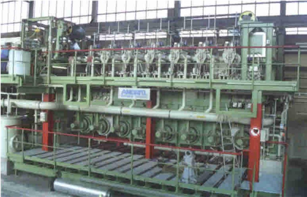
**Fig. 13** A smaller electrogalvanising addition to an existing coil coating plant
