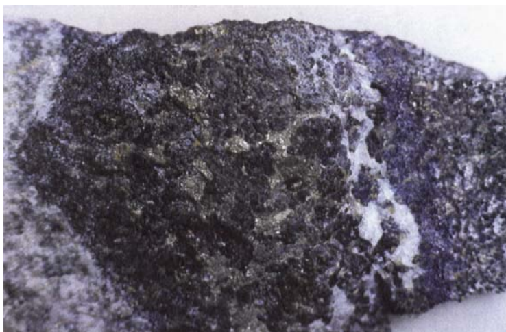
Fig. 3 Slab of a typical piece of the Merensky Reef, Rustenburg section (Amplats). Note the thin chromitite layer (black, approximately 1.5 cm thick) outlining the bottom contact of the reef, as well as the coarse-grained (pegmatoidal) nature of the reef. The white rock (norite) consists predominantly of plagioclase feldspar. The bright spots are the sulfides. The footwall is on the left and the hanging wall is on the right
