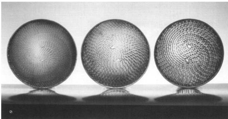
*Although less commonly used than their ceramic (cordierite) counterparts, metal catalyst substrates have been used in automotive applications for many years. Manufacturing techniques have been developed to produce them in very high cell density forms using extremely thin metal foil*
