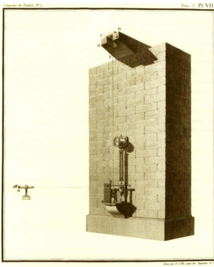
Fig. 2 The pendulum apparatus which Lenoir constructed at the Observatory in Paris. It has a fine iron wire holding a platinum sphere in front of the pendulum of a beating clock. By means of the telescope on the left an observer can follow the movement. The apparatus was enclosed in an airtight case (14)
