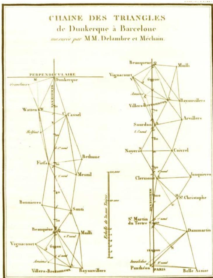
to measure the base lines, each approximately 36,000 feet long and requiring about 3,000 movements of the platinum rods. At each movement two rods had to be precisely aligned, put in exact contact by adjustment of the sliding tongue on one of them, and then measured. Wherever possible the corners of the triangles were high points such as hilltops or church towers, and all the measured distances had to be corrected to allow for variations in height and the curvature of the Earth.
