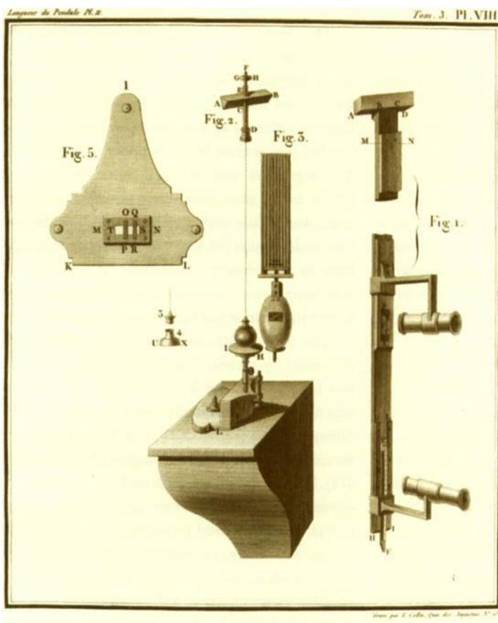
Fig. 3 Some parts of the pendulum apparatus. The measuring scale is on the right. (Fig. 1). The metallic thermometer can be read through the upper microscope, while the vernier on the platinum scale can be read through the lower microscope (14)
