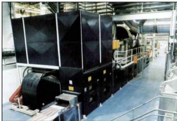
*The oven recovers waste heat for efficient energy use. Advanced materials handling techniques and pollution suppression devices maximise yields and eliminate wastage*
