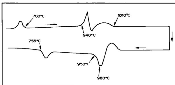
Fig. 2 DTA curves of titanium alloy 10Ni-20Ru ( $\delta+\eta+\beta$ ) and reference alloy 20Ni-80Ti ( $\eta+\beta$ ). On heating, melting begins at ~ 940°C for 20Ni-80Ti, and near the peak of the curve for 10Ni-20Ru; at 1010°C solid-liquid state reactions end. On cooling, crystallisation begins at ~ 1020°C for 10Ni-20Ru and at ~ 1000°C for 20Ni-80Ti. At 980 and 950°C, respectively, the solid-liquid reactions end. At 700 (20Ni-80Ti) and 755°C, solid state reactions occur for Ti-based alloys
