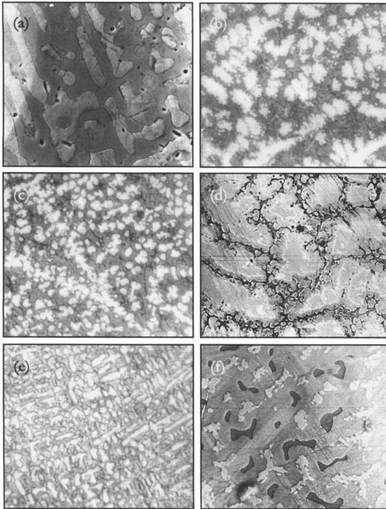
Fig. 3 SEM microstructures of the Ti-TiNi-TiRu alloys:
