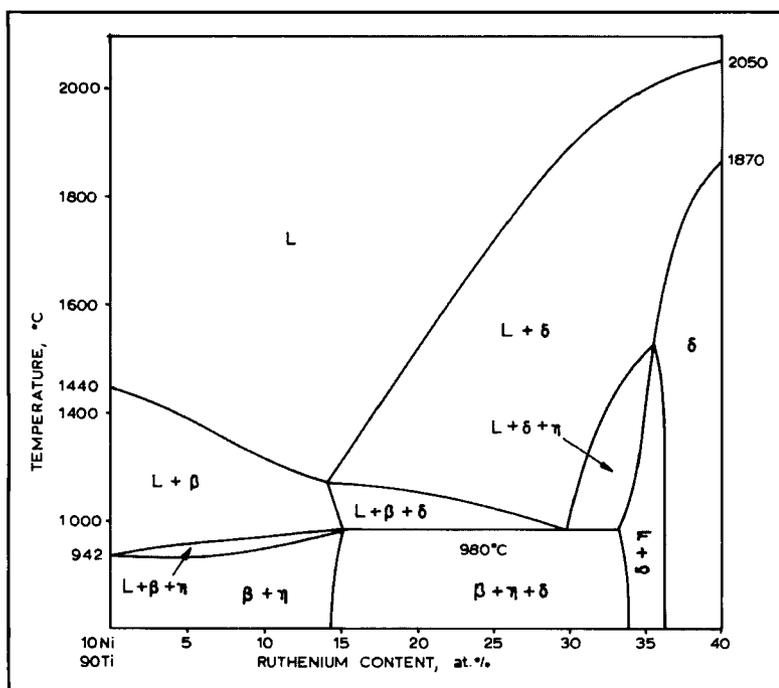
The large temperature range of the  $\delta$ -phase primary crystallisation and the very narrow one for the following  $L \leftrightarrow \eta+\beta$  reaction results in non-equilibrium proportions of the phases present (Figures 3d and 4). On subsequent annealing, the 10Ni-20Ru alloy becomes a three-phase alloy (Figure 3f).
