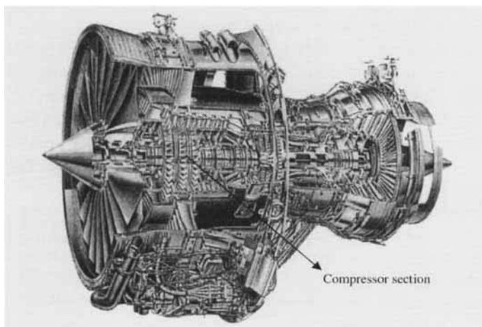
*Fig. 1 Mechanical arrangements of a modern gas turbine engine showing the compressor sections where titanium alloys are used*
