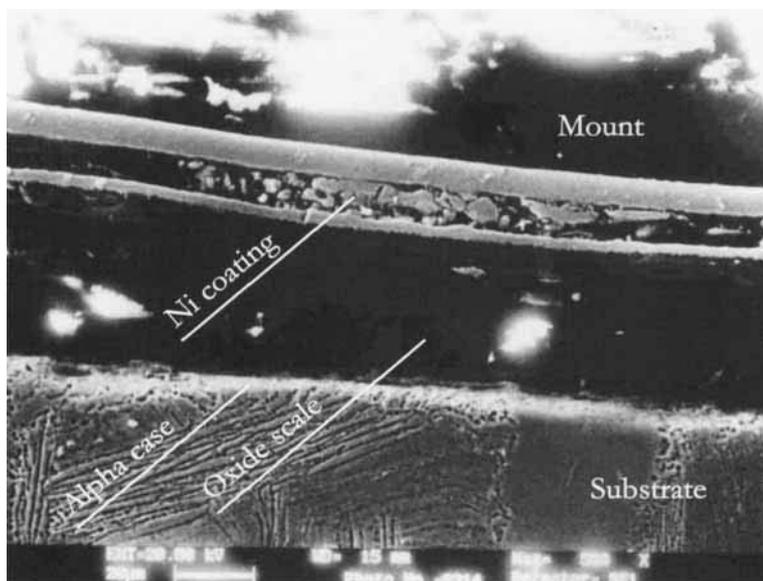
(7). However, the coating method for the titanium alloys is different from that used for the nickel-based superalloys.
