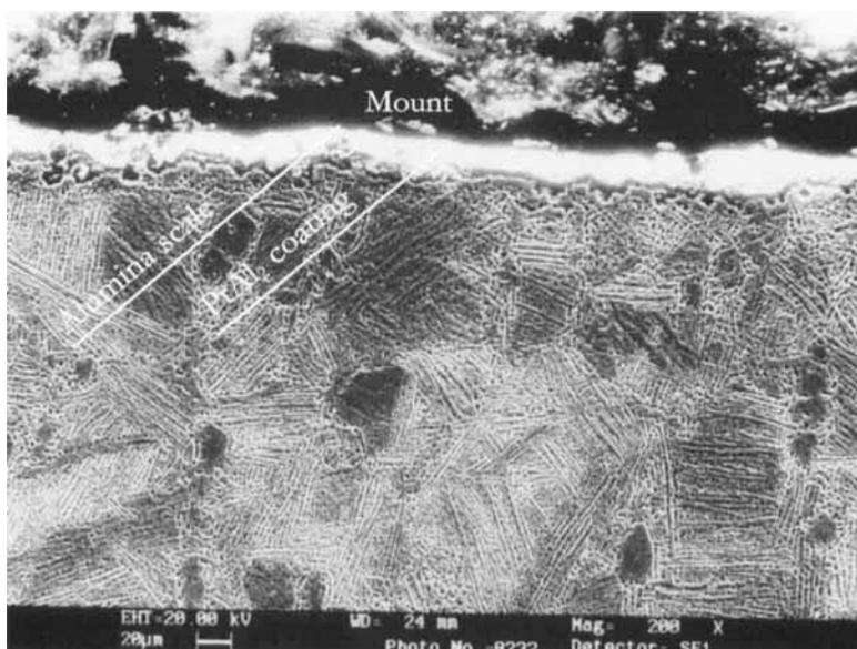
*Fig. 3 Scanning electron micrograph showing the presence of a protective alumina scale on the surface of the platinum aluminide coating after oxidation at 800°C in air for 400 hours*
