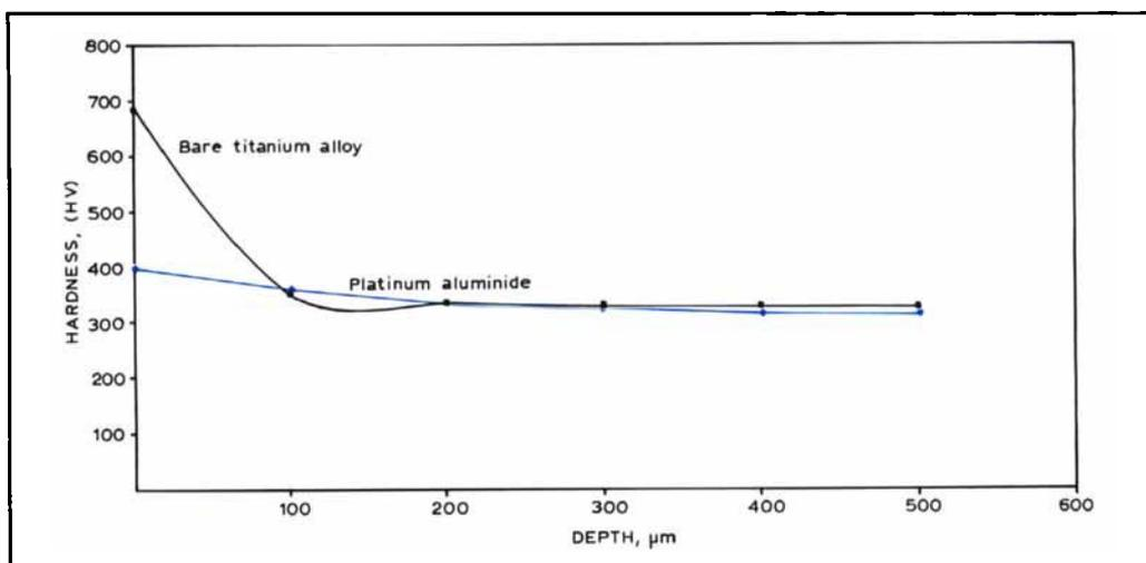
Fig. 5 Microhardness profiles of bare titanium alloy after cyclic oxidation at 800°C for 100 hours, and of platinum aluminide coated titanium alloy after cyclic oxidation at 800°C for 400 hours. There is an extensive hardened zone for the uncoated alloy but not for the coated alloy
