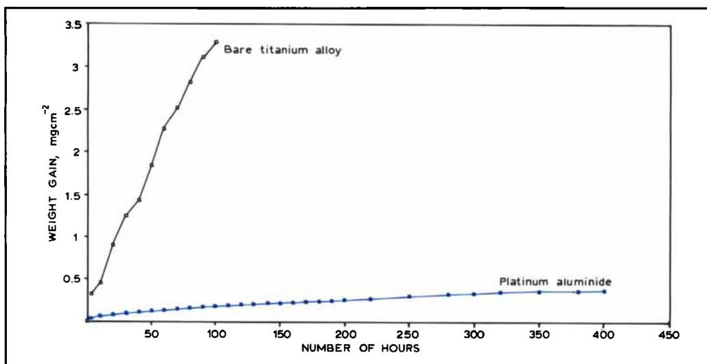
Fig.2 Cyclic oxidation kinetics at 800°C of the titanium-based alloy, IMI 834, with and without a platinum aluminide coating. The superior performance of the coating reduces the weight gain of the titanium alloy
