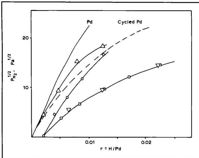
Fig. 7 Dilute phase  $H_2$  isotherms (taken at 273 K) for an internally oxidised (1073 K, 72 h)  $Pd_{0.97}Al_{0.03}$  alloy:
