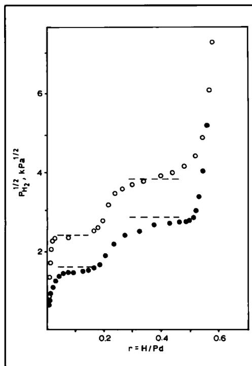
Fig. 6 H<sub>2</sub> isotherm (323 K) for a partially internally oxidised Pd<sub>0.97</sub>Al<sub>0.03</sub> alloy. The lower set of horizontal dashed lines are plateau pressures for the oxidised part of the alloy, Pd-H. The upper set of horizontal dashes are for the unoxidised Pd<sub>0.97</sub>Al<sub>0.03</sub> alloy. o absorption of H<sub>2</sub>; ● desorption of H<sub>2</sub>.
