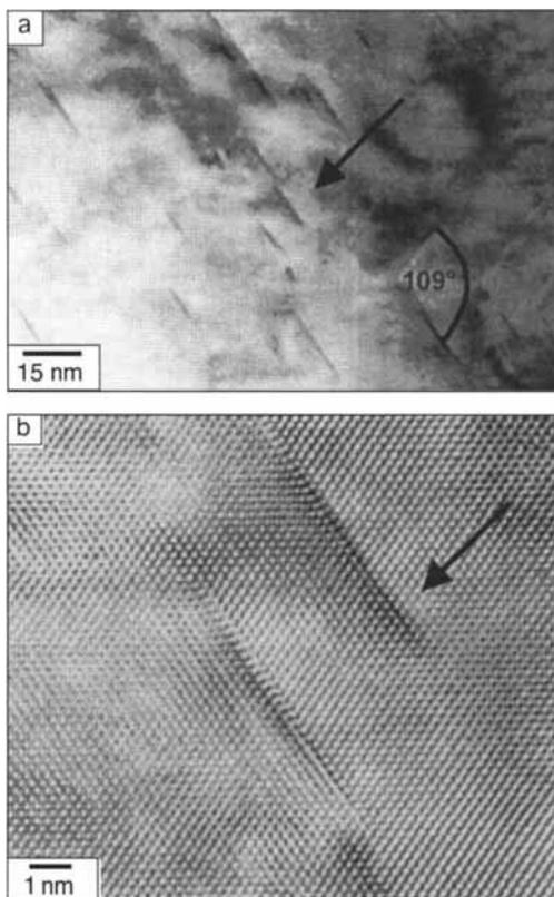
Fig. 12 HREM images for a  $Pd_{0.80}Pt_{0.20}$  alloy after treatment with  $H_2$  at 100 MPa for 3 h at 673 K. Two different magnifications are shown in (a) and (b). The illumination is parallel to the [011] zone axis. Before the  $H_2$  treatment, the lattice appears to be perfect (61)
