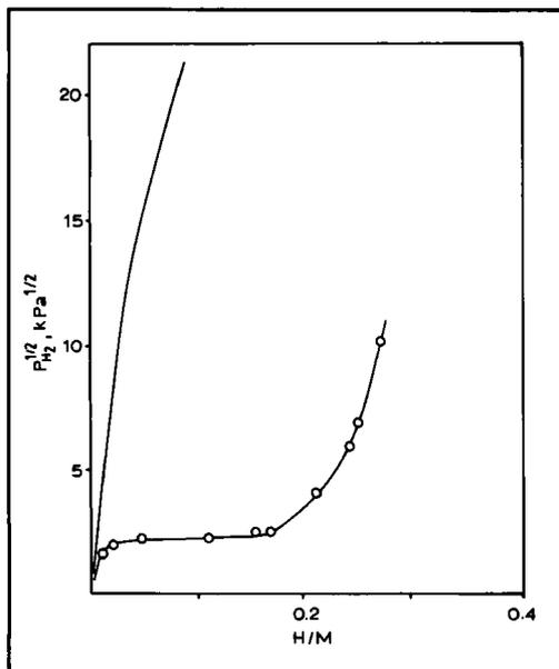
Fig. 11  $H_2$  isotherms (273 K) for a  $Pd_{0.80}Pt_{0.20}$  alloy. Continuous line is for the homogeneous alloy;  $\circ$  after treatment in 100 MPa  $H_2$  for 3 h at 673 K (redrawn from (59))
