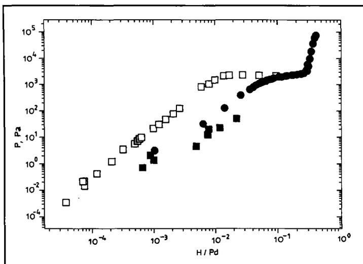
Fig. 13 Experimental solubility data at 310 K for  $H_2$  solubility in a 3.1 nm Pd cluster. Open symbols indicate absorption; filled symbols indicate desorption (68)
