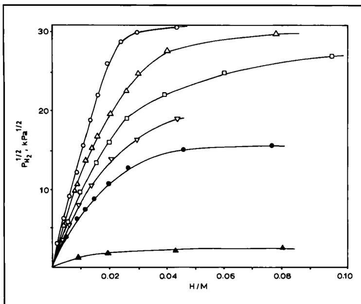
Fig. 10 Dilute phase  $H_2$  solubilities (303 K) for a  $Pd_{0.80}Rh_{0.20}$  alloy cooled from  $\approx 1100$  K at different rates or heat treated in vacuo at 873 K or in  $H_2$  (100 MPa).
