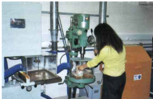
An employee at the Johnson Matthey Shanghai autocatalyst plant takes a core sample from a production catalyst for quality control tests
