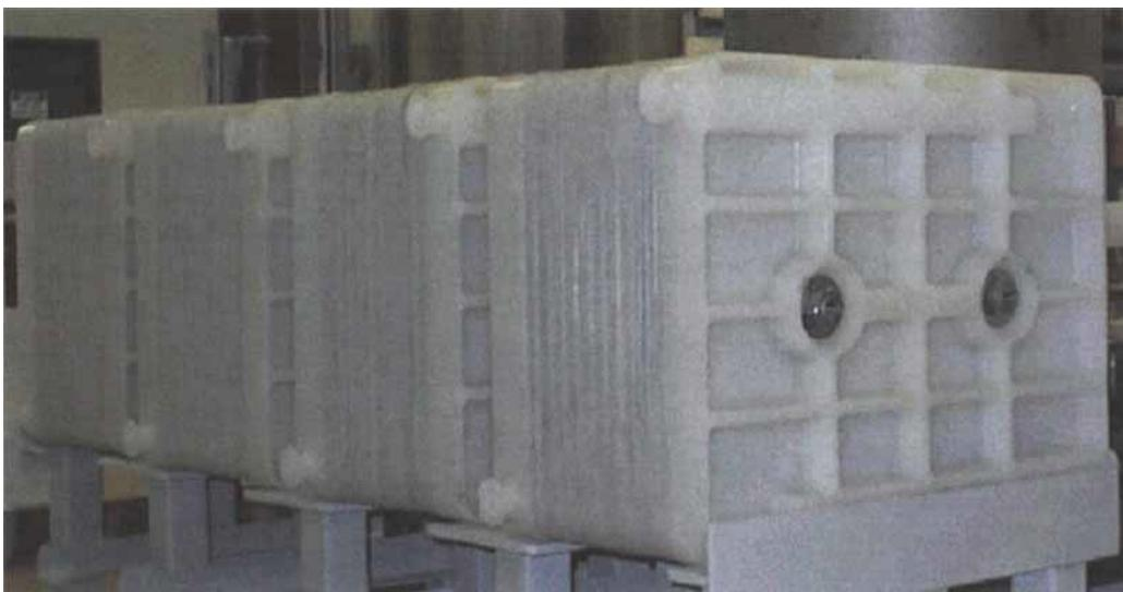
*Fig. 1 Four welded CerOx electrochemical T-Cells manufactured for the System 4 delivered to the University of California at Irvine to be used for organic waste destruction. Each T-Cell has 10 platinum-plated electrodes which are electrically connected in series*
