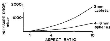
Pellets must be physically strong and resistant to attrition losses (dusting). An increasing pressure drop indicates pellet disintegration and can result in a deteriorating catalyst performance.
