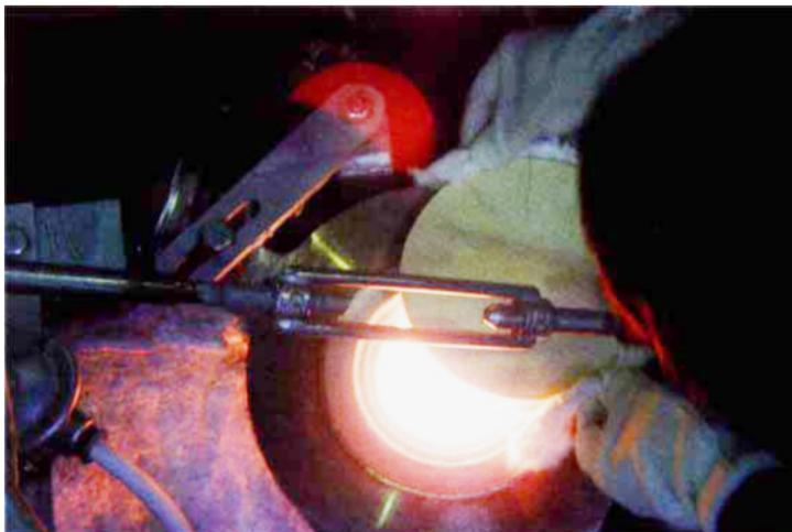
Power Coatings™ systems, such as that used by Crystalex, Nový Bor, Czech Republic, is less than 0.2 per cent. This tightly-controlled delivery weight contributes towards the increased quality of the product and to a reduction in the rejection rate by ensuring that the correct weight of glass is consistently transferred to each mould, thus facilitating smooth, efficient operation of the glass forming machines.
