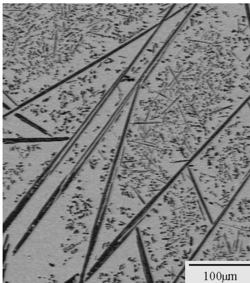
Fig. 7 Scanning electron micrograph, backscattered mode, of the 50.6 Pt-22.1 Al-27.3 at.% Ru sample after arc-melting. The light matrix is Pt<sub>3</sub>Al and the dark phase (needles + fine dark phase) is the Ru-rich solid solution
