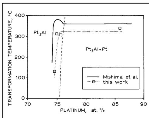
Fig. 4 Comparison of phase transformations detected in Pt<sub>3</sub>Al by DSC and/or DTA in the present work, with those reported previously by Mishima *et al.* (10)
