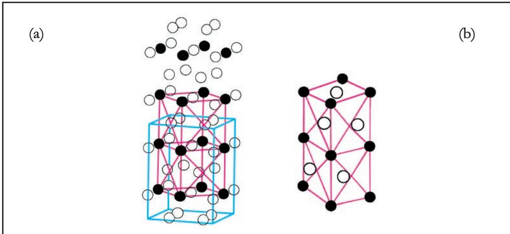
Fig. 1(a) The  $DO_c'$  unit cell (blue) of the  $Pt_3Al$  tetragonal structure (low temperature). It contains a distorted f.c.t. lattice which is also shown in (b). The Pt atoms (white) lie slightly offset from the centre of the faces and the Al atoms (black) sit at the corners of the cell. In (b), for clarity, only the Pt atoms on the top and front faces are shown
