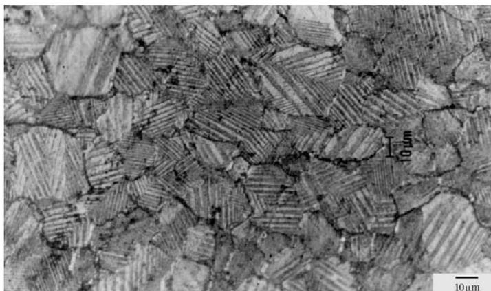
diffuse out of the matrix and into the Pt-rich solid solution. For larger additions of Ru, a mixture of cubic Pt<sub>3</sub>Al and a h.c.p. (hexagonal close packed) Ru-rich solid solution containing Pt was observed, see Figure 7. After heat treatment, there was minimal Ru dissolved in the Pt<sub>3</sub>Al matrix and minimal Al in the Ru-rich solid solution.
