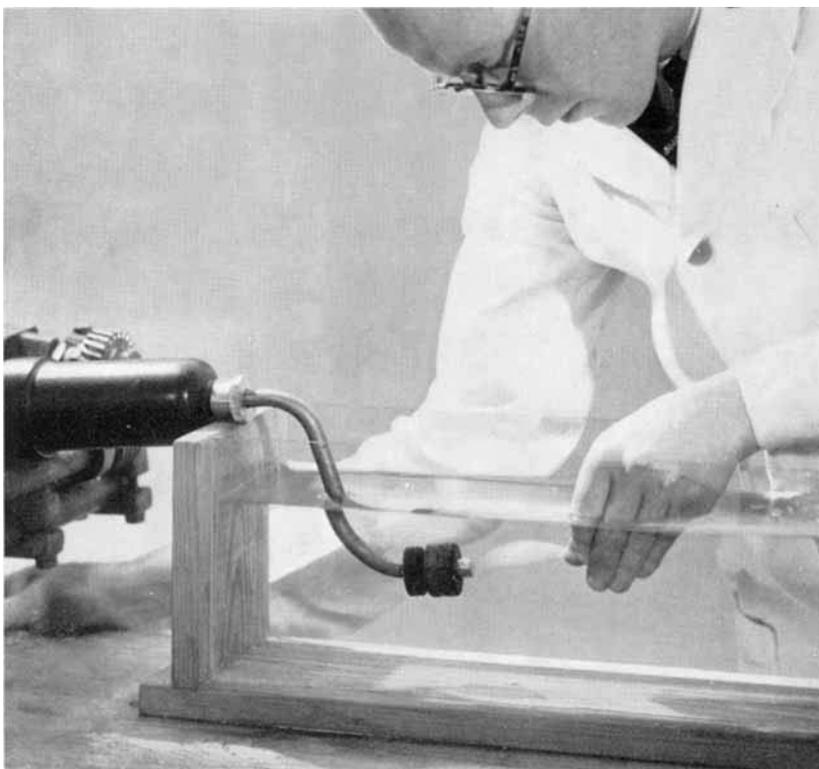
*A simple demonstration of the formation of a multi-filament yarn by pumping viscose solution through the holes in a jet immersed in an acid bath (Courtaulds Ltd)*
