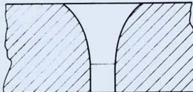
*In addition the capillaries of each of several thousand orifices in one jet must all be of exactly the same length, while the orifices themselves must be highly polished and truly circular. Johnson Matthey jets are produced to meet these stringent requirements*
