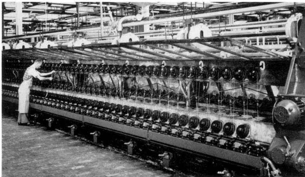
*Many thousands of platinum alloy spinning jets are in use in a modern viscose rayon plant. The illustration shows one unit engaged in spinning continuous filament in a Courtaulds factory*
