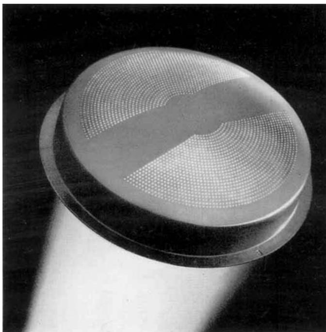
*The number of holes and their pattern in a jet vary according to the type of rayon to be produced. This type of platinum-gold alloy jet has over 2,000 orifices and is made and used in the production of staple fibre by Courtaulds Ltd*
