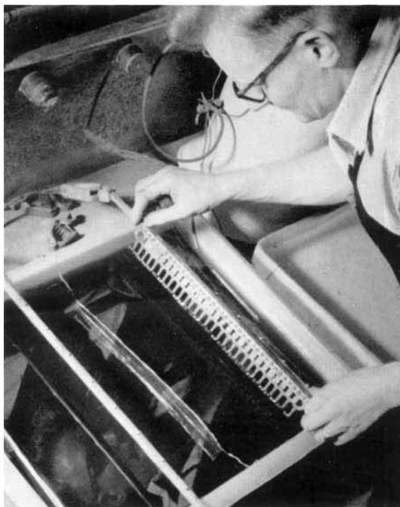
*Rhodium plating a batch of electrical contact springs*
