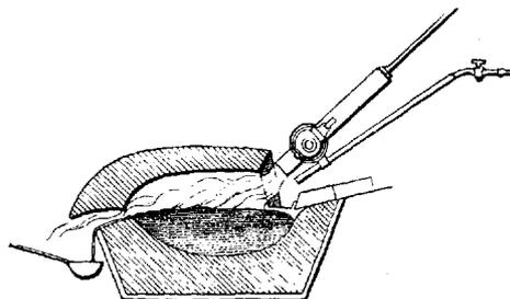
*Removing the litharge in a fused state from the surface of the molten platinum*
