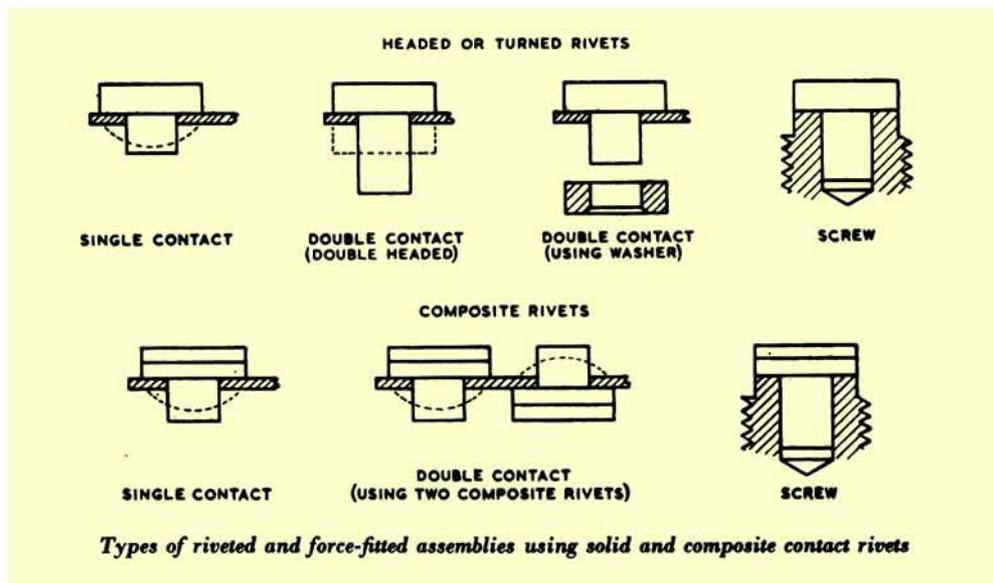
tact material rule out heading, the rivets must be produced by turning. In comparison with heading, turning is slow and produces swarf which must be returned for refining. Moreover, unlike the headed contact, the hardness of the head of a turned rivet is the same as that of the shank.
