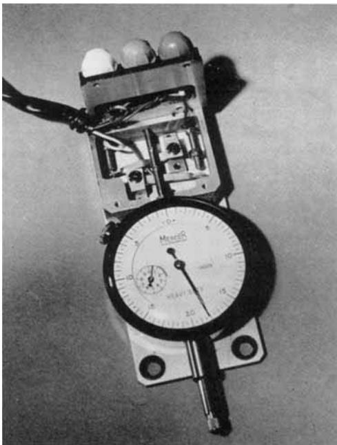
*The 10 per cent iridium-platinum alloy is used in this electric dial gauge by Thomas Mercer (Air Gauges) Limited. The moving contacts consist of rivets fitted into brass arms; the fixed contacts comprise fitted screws*
