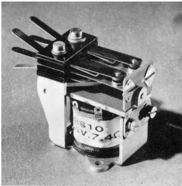
*An example of the use of 40 per cent silver-palladium rivets is found in this light duty relay by Waymouth Gauges & Instruments Ltd*
