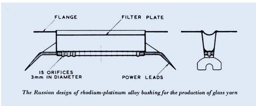
diagram of this design of bushing, having fifteen orifices each 3 mm in diameter, is reproduced here.
