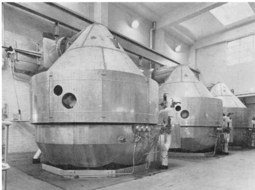
*The three ammonia converters installed at Ardeer. Each converter has three rhodium-platinum catalyst gauzes, 114 in. in diameter, woven by Johnson, Matthey & Co., Limited*
