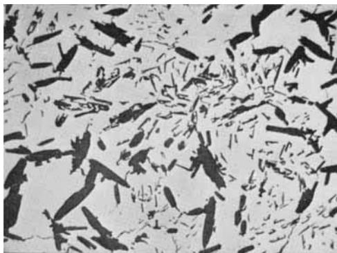
*Microstructure of 20 per cent samarium-palladium alloy after treatment in air at 1200°C for 100 hours*
