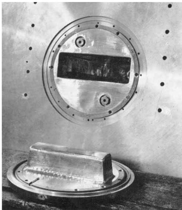
*The platinum-lined muffle and door of one of the new fluorination furnaces*
