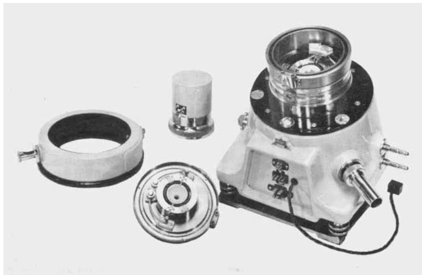
The Unicam S.150 high temperature X-ray diffraction camera, dismantled to show the platinum furnace assembly
