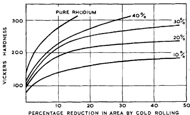
Fig. 14 Work hardening curves of rhodium-platinum alloys (Reference 41)
