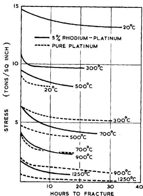
Fig. 13 Creep properties of pure platinum compared with those of the 5 per cent rhodium-platinum alloy at temperatures between 20 and 1250°C (Reference 43)
