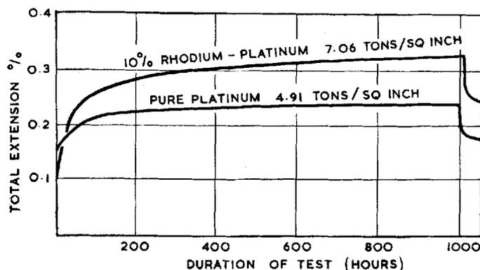
Fig. 12 Room temperature creep curves of pure platinum and of the 10 per cent rhodium-platinum alloy (Reference 42)
