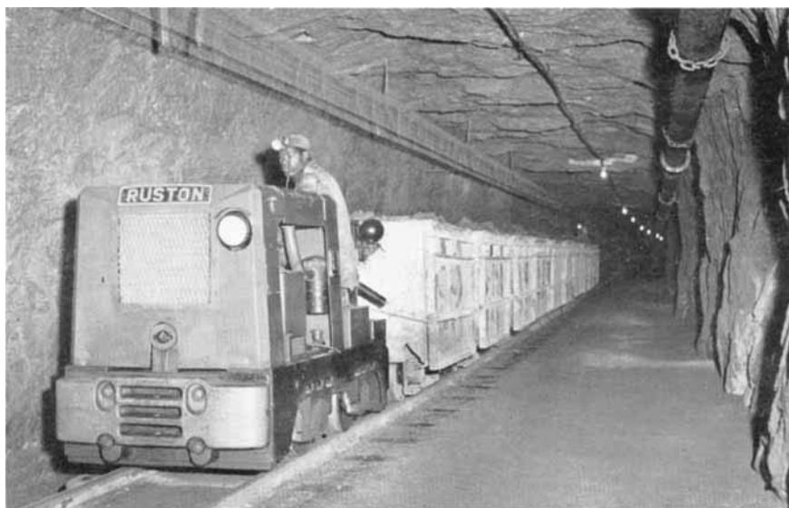
*From the central scraper gully, ore is loaded into hopper trains and delivered to the shaft box*
