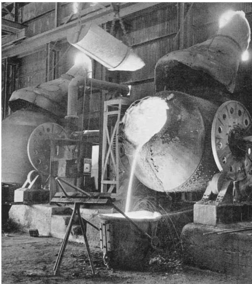
*Pouring blown matte from one of the Great Falls converters. After cooling and breaking up, the matte is shipped to Johnson Matthey for the extraction of copper, nickel and the six platinum metals*
