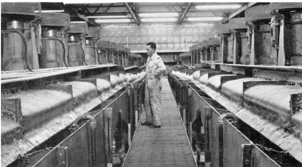
*Part of the flotation plant at Rustenburg. Eight banks of eighteen cells act as roughers, with a further two banks of eighteen cells as cleaners*
