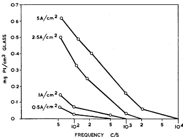
*The colloidal dispersion of platinum in a heavy crown glass as a function of frequency for various current densities. Temperature 1290°C, duration of test 30 minutes. At 10 kilocycles per second measurable dispersion of platinum from the electrodes ceases.*
